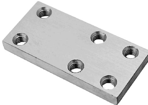
The Long D Plate (Part # S9002) is made of 316 stainless steel and fastened to the back of a multi-cylinder HD Series Type D interlock to allow front mounting (see HD Series Data Sheet 1.4). The thickness of the Long D Plate is 3/8". To order this plate with your multi-cylinder HD Series Type D interlock, put the letter "P" in column fourteen of the interlock part number - reference the HD Series Ordering Guide.
