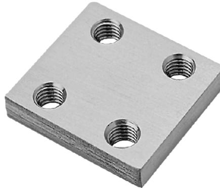
The Short D Plate (Part # S9001) is made of 316 stainless steel and fastened to the back of a single cylinder HD Series Type D interlock to allow front mounting (see HD Series Data Sheet 1.4). The thickness of the Short D plate is 3/8". To order this plate with your single cylinder HD Series Type D interlock, put the letter "P" in column fourteen of the interlock part number - reference the HD Series Ordering Guide.
